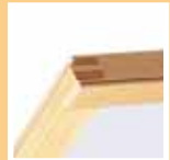
Sash double-mortise and tenon joint
